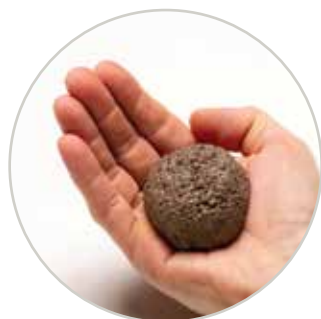
Too much moisture
